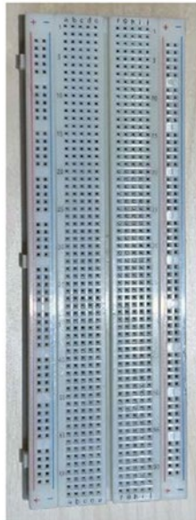
Figure 21-3. A breadboard for prototyping electronic circuits
