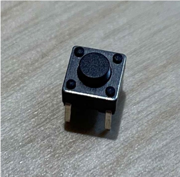
Figure 21-8. A simple push-button tact switch
