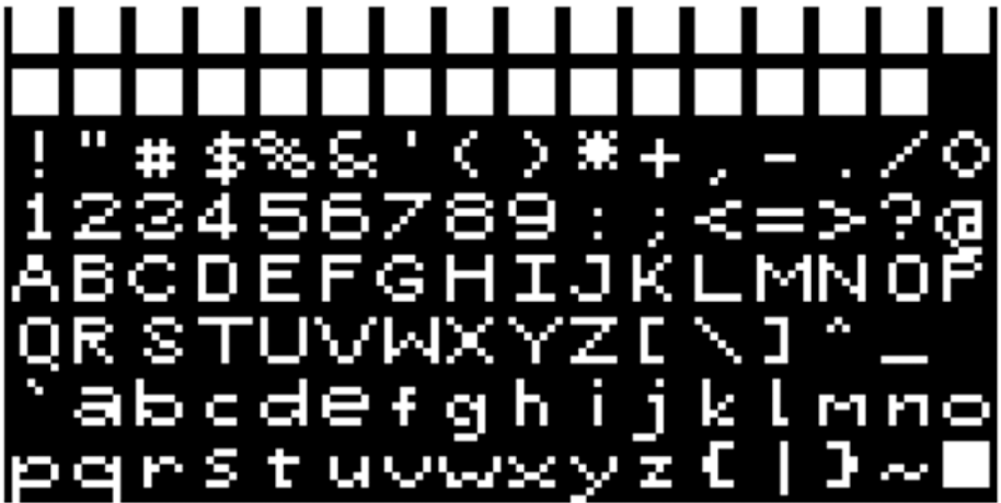
Figure 20-3. Example of a bitmap font taken from https://opengameart.org/content/8x8-ascii-bitmap-font-with-c-source
