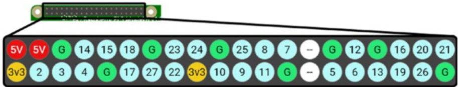
Figure 21-17. The position of each GPIO, voltage, and ground pins
